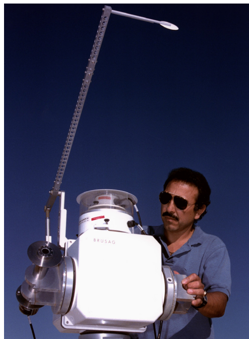
SNL technician examines a solar tracker that follows the sun. The tracker shown is part of SNL's Atmospheric Radiation and Cloud Station (ARCS) outdoor sensor array. This is part of DOE's ARM program, which is seeking to find how sunlight and infrared radiation interact with clouds and, in particular, whether varying levels of atmospheric moisture could influence Earth's radioactive energy to the point of causing long-term global climate changes.
